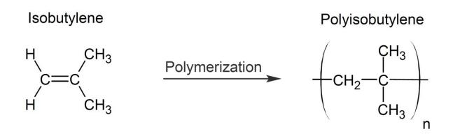
It is produced by cationic polymerization of isobutylene using  $BF_3$  and  $AlCl_3$  catalyst in a suitable solvent such as hexane or methylene dichloride at -80°C. The polymer dissolves in many hydrocarbons. Polyisobutylene is chemically one of the most inert polymers known so far. Moisture, acids, and alkalis have practically no effect on this polymer.
