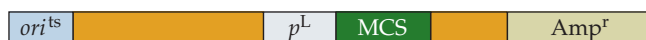
FIGURE 6.6 Linear representation of E. coli expression vector pCP3 with a temperature-sensitive origin of DNA replication ( ori^{ts} ) that causes an increase in the plasmid copy number at 42°C and a p^L promoter controlled by a temperature-sensitive repressor protein, a multiple cloning site (MCS), and an ampicillin resistance ( Amp^r ) gene.
